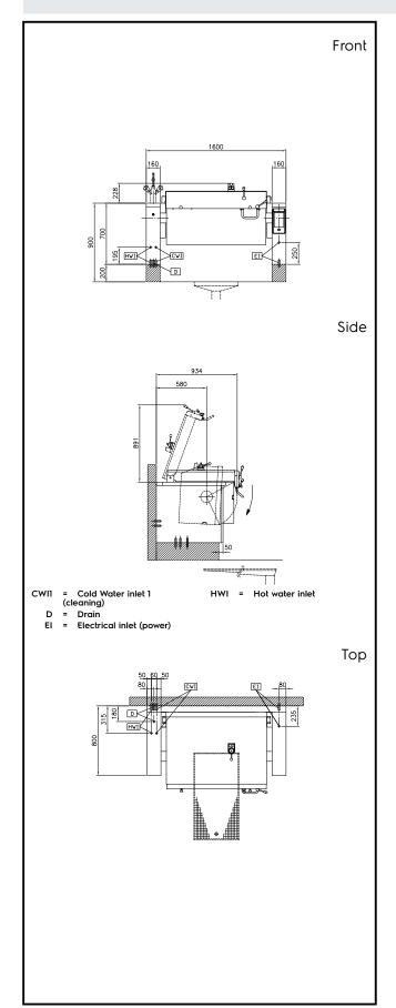
Electric 400 V/3N ph/50/60 Hz Supply voltage: Total Watts: 20.6 kW Installation: FS on concrete base;FS on feet;On base;Standing Type of installation: against wall **Key Information:** Working Temperature MIN: 50 °C Working Temperature MAX: 250 °C Vessel (rectangle) width: 1050 mm Vessel (rectangle) height: 209 mm Vessel (rectangle) depth: 558 mm External dimensions, Width: 1600 mm
